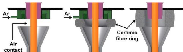
Figure 5: Concepts to protect the pouring stream during ingot casting (schematic) /4/
