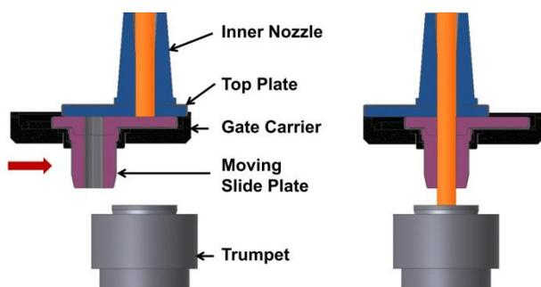
Figure 3: Schematic drawing of a sliding gate valve with two refractory plates
