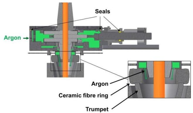
Figure 7: Schematic drawing of the new developed gas-tight sliding gate
