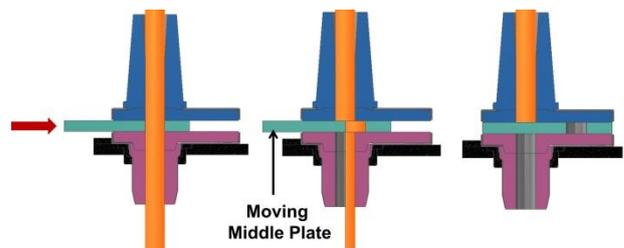
Figure 4: Schematic drawing of a sliding gate valve with three refractory plates
