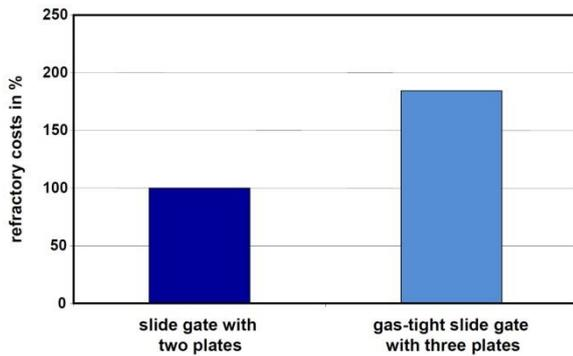
Figure 9: Refractory costs of a gas-tight slide gate with three plates in comparison to a slide gate with two plates
