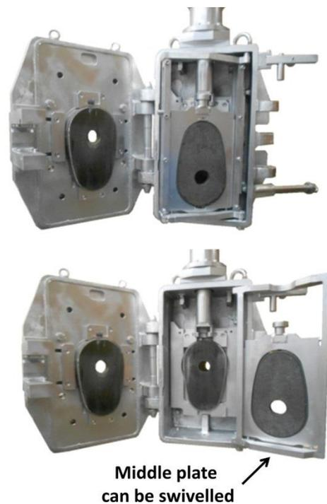
Figure 8: New developed FT3 160GT slide gate
