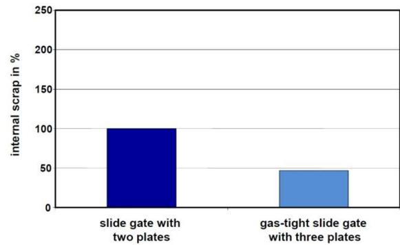
Figure 11: Influence of the slide gate system on the internal scrap (subsurface non-metallic inclusion, detected by ultrasonic testing)
