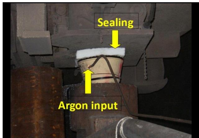
Figure 6: Pouring stream protection during ingot casting /5/
