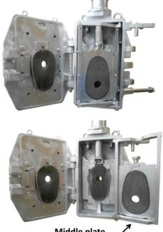
Middle plate / can be swivelled Figure 8: New developed FT3 160GT slide gate
